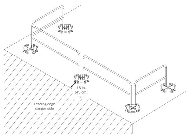
Rail sections are kept securely in place simply by inserting a lockpin
